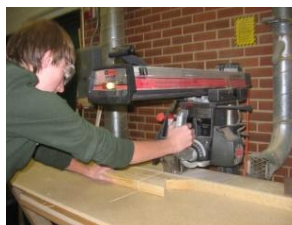
Wyatt Carter cutting his lumber to correct size on the new Radial Arm Saw.
